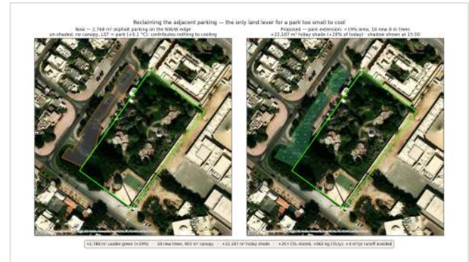
Fig. 27. Converting the adjacent NW parking lot: +18.8% area and +28% shade, next to Tier-A cluster #113.
