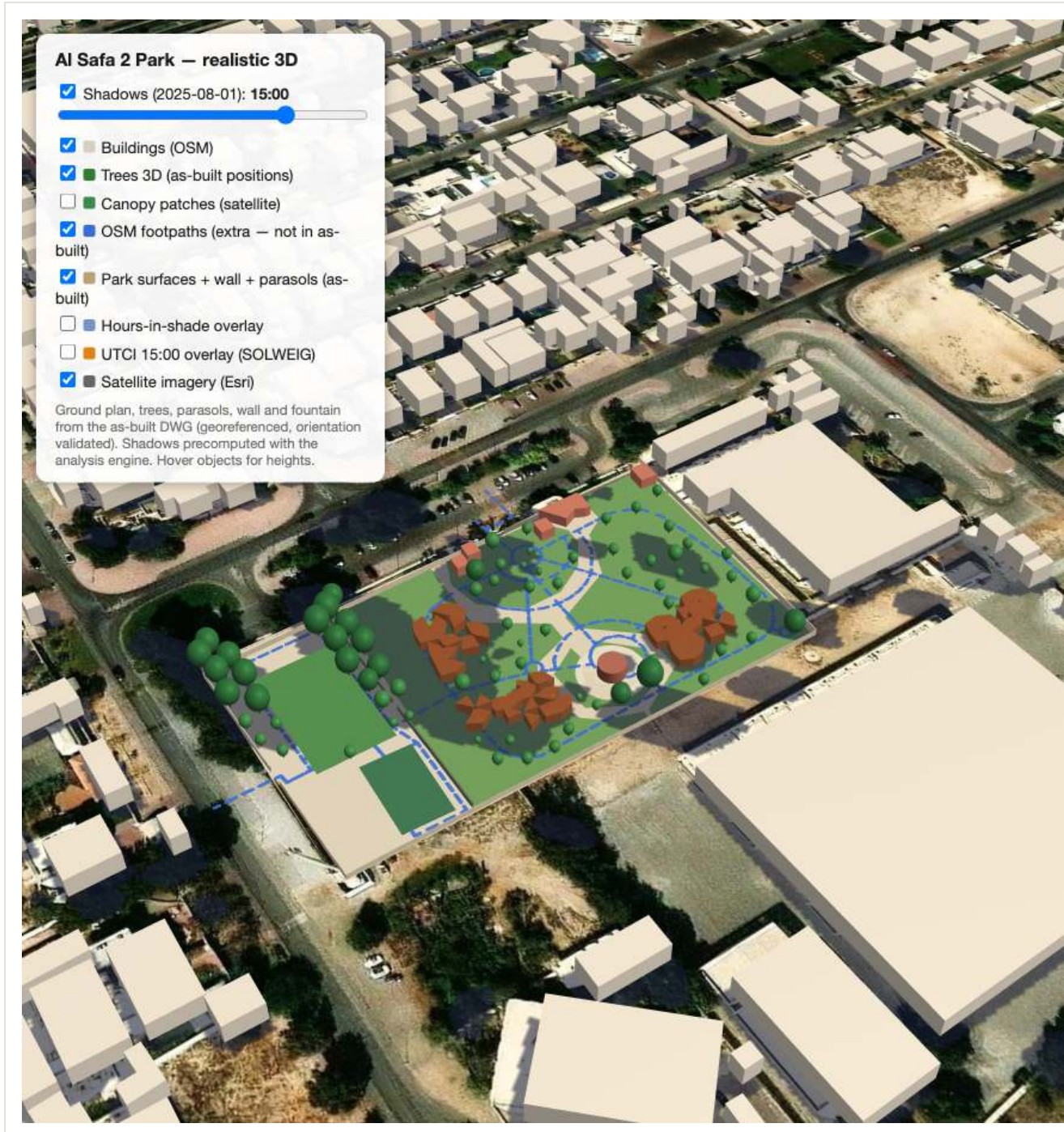
Fig. 1. The interactive 3D explorer: OSM buildings, 214 satellite-derived canopy patches, the as-built ground surface and 68 parasols on Esri imagery, with design-day shadows for 2025-08-01.
