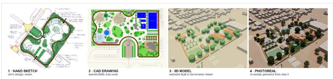
Fig. 19. Sketch → CAD → 3D model → AI restyle. Step 2 shows the layered DWG for proposal 2 while steps 1, 3 and 4 are proposal 1, so this illustrates the stages rather than one unbroken
